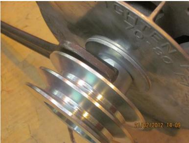
Use the torque wrench and 24mm socket and torque the shaft nut to 70-80 ft lbs (95N.m - 108N.m)
